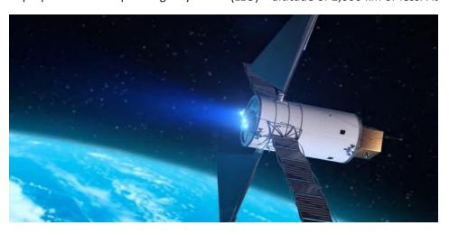
An air breathing thruster could keep a satellite operational for extended periods of time if it only uses the air around it for fuel instead of propellants. An air-breathing engine works by collecting the sparse air at the edge of the atmosphere and compresses it to a point that it becomes thermalisedionised plasma. It then fires out the plasma using an electric charge to achieve thrust.
