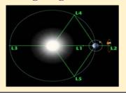
a body to remain relatively stationary Types: There are five Lagrange Points, denoted as L1, L2, L3, L4, and L5.
